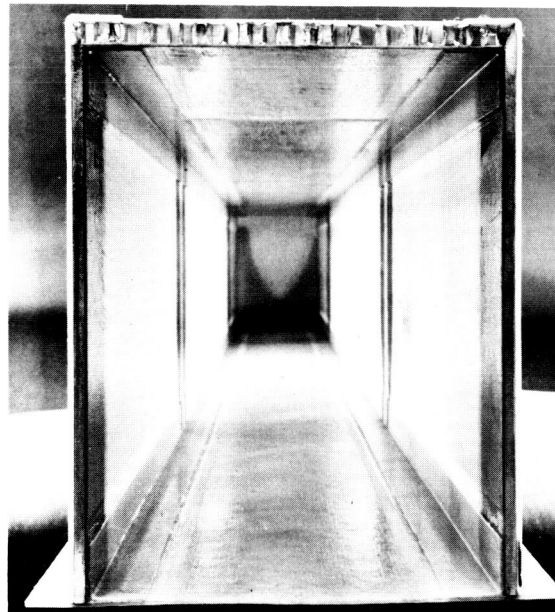
Figure 2. End View of a Completed Fiberglass Reinforced Box Beam
