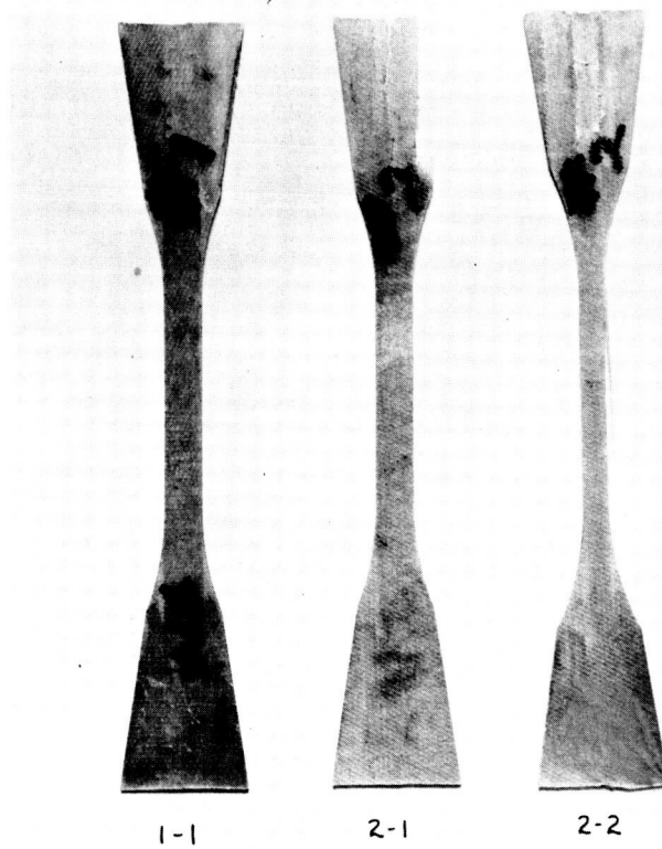
Figure 19. Dogbone Tensile Test Specimens Showing Failure in the Area of the Holding Jaw
