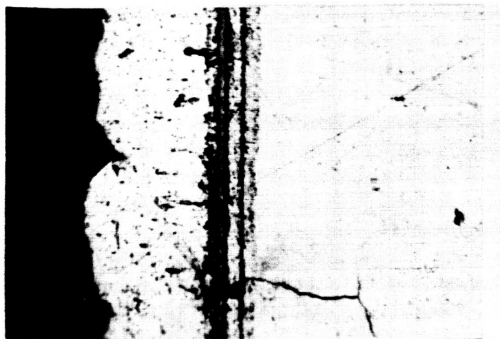
Figure 16. First Sign of Failure during Microbend Test of Columbium-Plated Iridium Annealed Eight Hours at 1350°C. Mag. 500 X, N-6821
