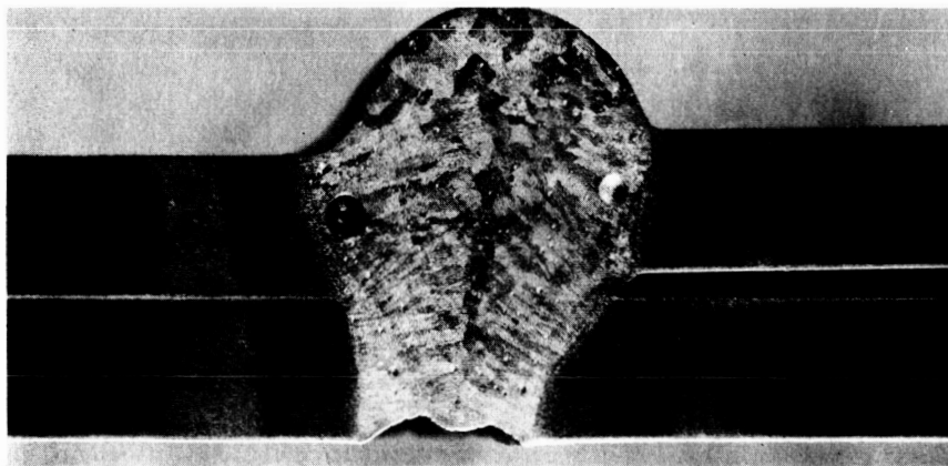
B. 0.030-IN. GAP BETWEEN TEST PART AND BACKING STRIP NOTE: UNDERBEAD SUCKBACK, LARGE VOIDS, AND SCATTERED MICROPOROSITY
