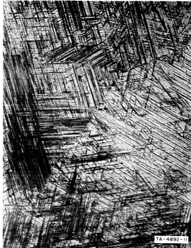
FIG. 2 STRUCTURE OF ARC MELTED TANTALUM CARBIDE BOULE NEAR ELECTRODE (500 X)
