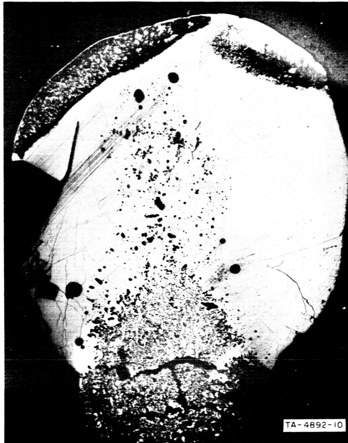
FIG. 1 VERTICAL SECTION OF A TANTALUM CARBIDE ARC-MELTED BOULE - heavily etched to show grain structure (26 X)
