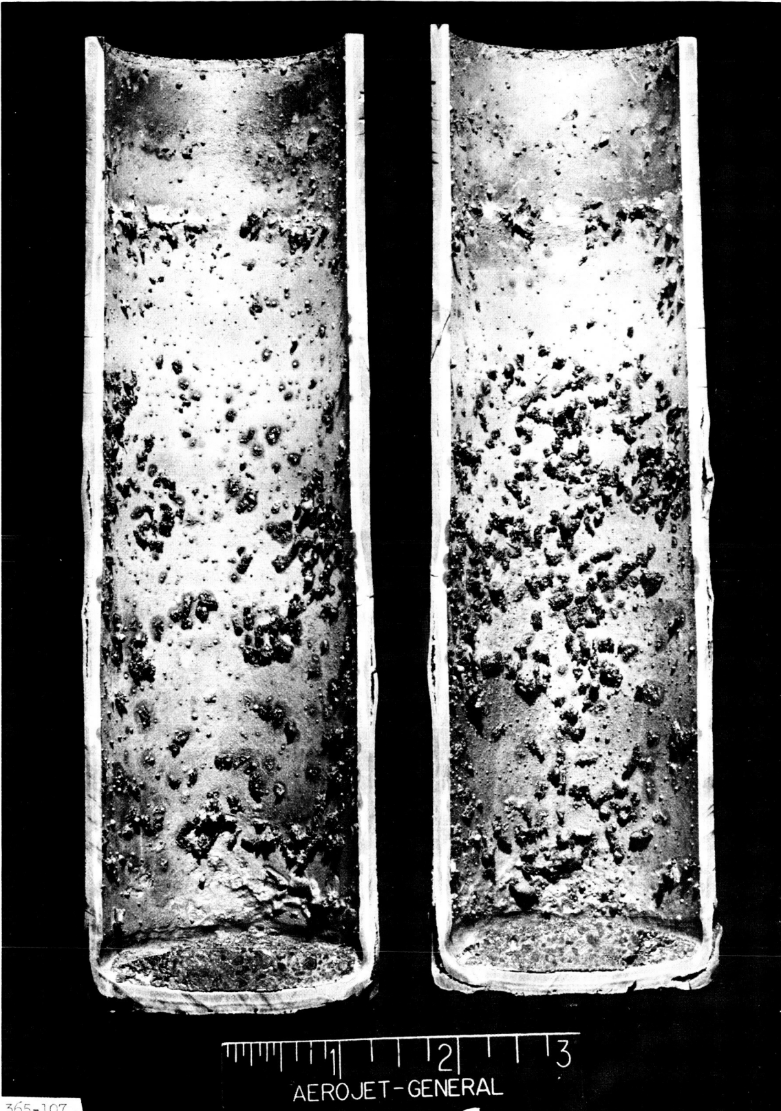
Inside View of Zirconia Crucible from Run 6 (large metal slug at bottom of crucible showed the following analysis: Si, 62.4; Fe, 23.5; Al, 5.8; Mn, 5.8; Ti, 1.3; Mg, 0.8; and Cu, 0.4)
