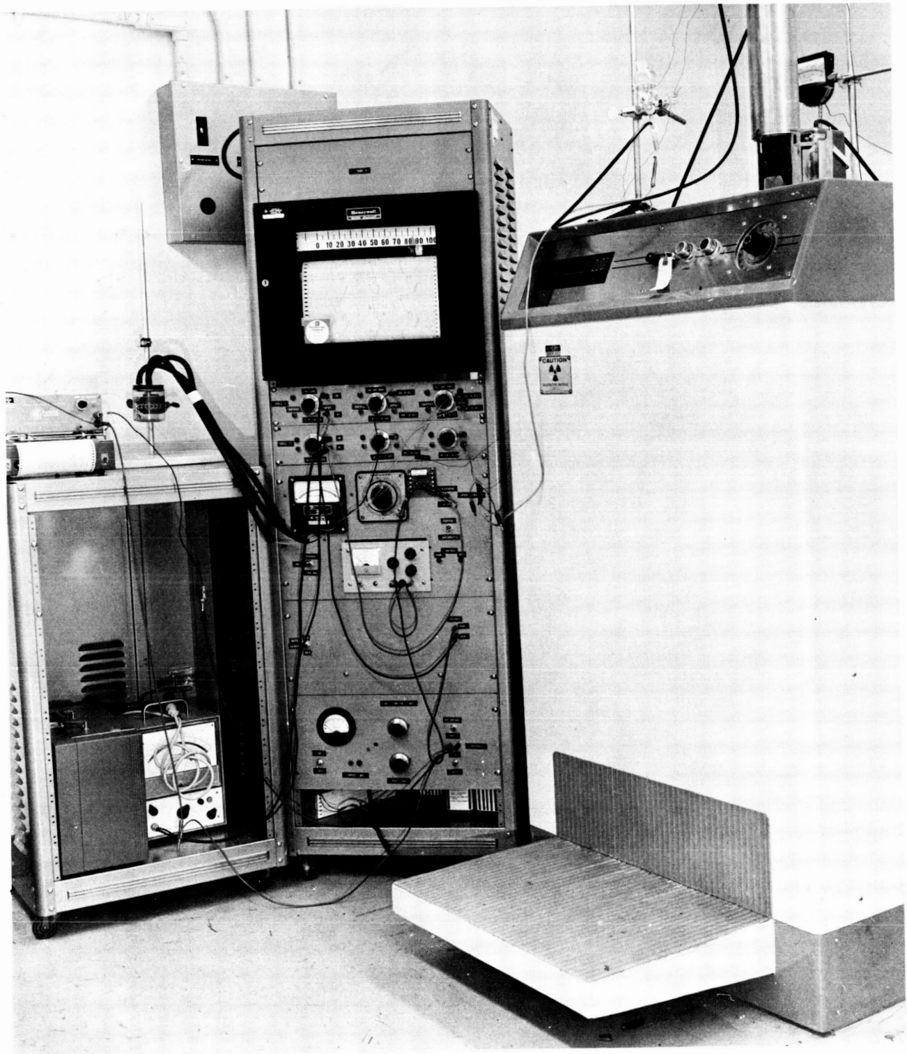
Figure 8. Test Cell Installed in NAA Science Center Co 60 Source.
