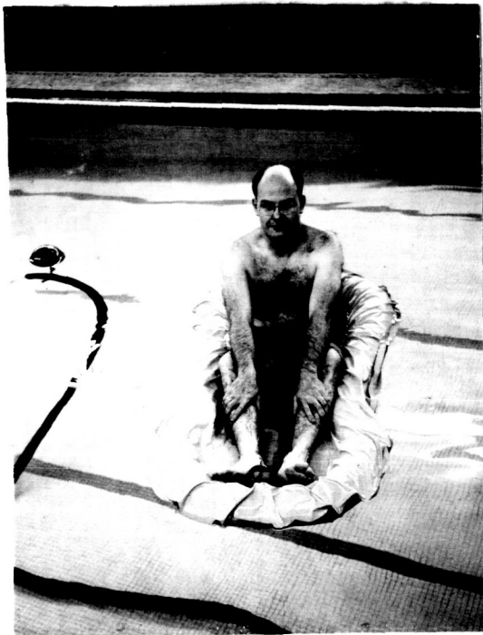
Figure 15 Raft with Inner Tube Inflated and Outer Tube Evacuated
