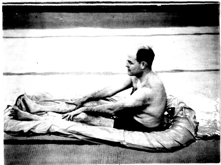
Figure 15 Raft with Inner Tube Inflated and Outer Tube Evacuated
