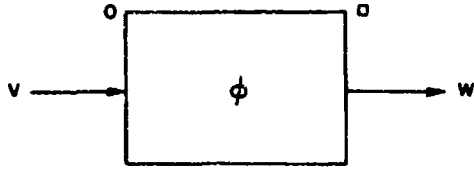
Fig. 1. Representation of a homomorphic system with input operation \circ , output operation \square , and system transformation \phi .
