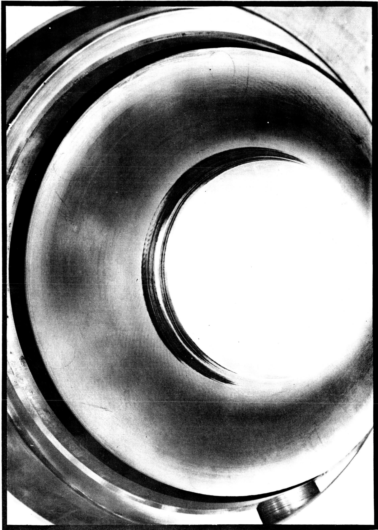
FIG 10 IMPELLER RUB MARKS IN PUMP SCROLL AFTER TEST IN PT-4 STAND
