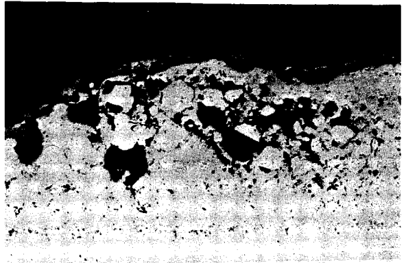
b) Section 1, TC 27 Superheater Outlet (Deposition)
