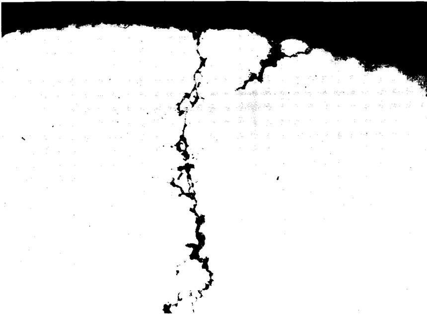
a) Section 6 Boiler Outlet (Cracking and Layer and Crevice Attack)
