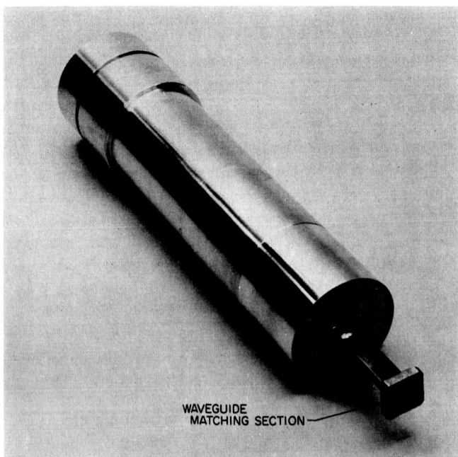
Fig. 11. 21.9-Gc JPL-fabricated gain standard horn
