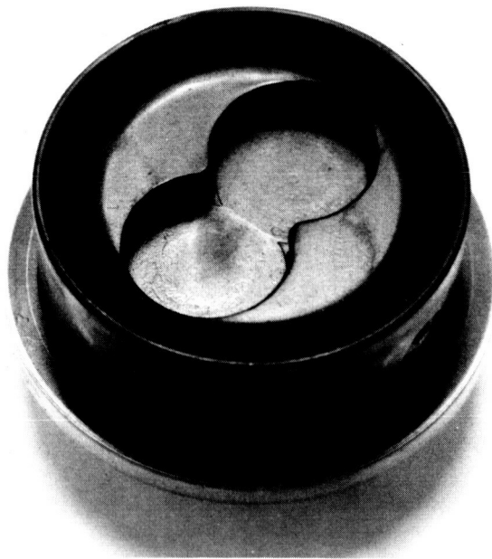
Fig. 3-25 - "Figure 8" Combustion Chamber
