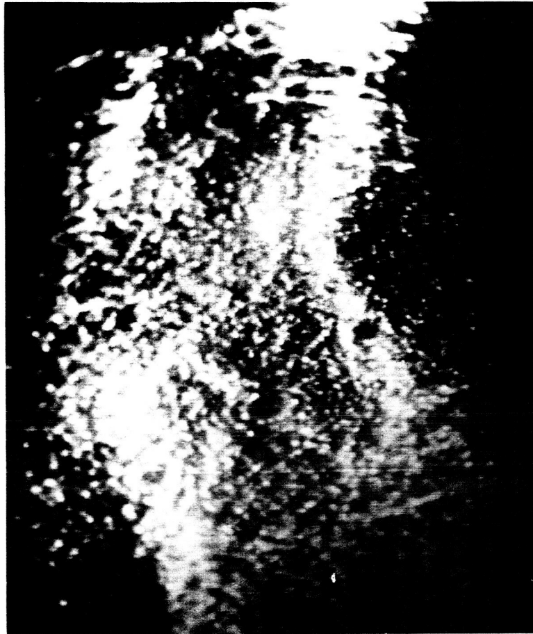
Fig. 6b. Same tip as in Fig. 6a after partial field evaporation. Streaks have disappeared and a large number of bright spots appear.
