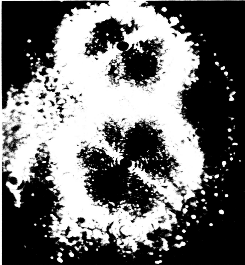
Fig. 7. Carburized C.P. tungsten heated as wire below the melting point in a nitrogen atmosphere and quenched.
