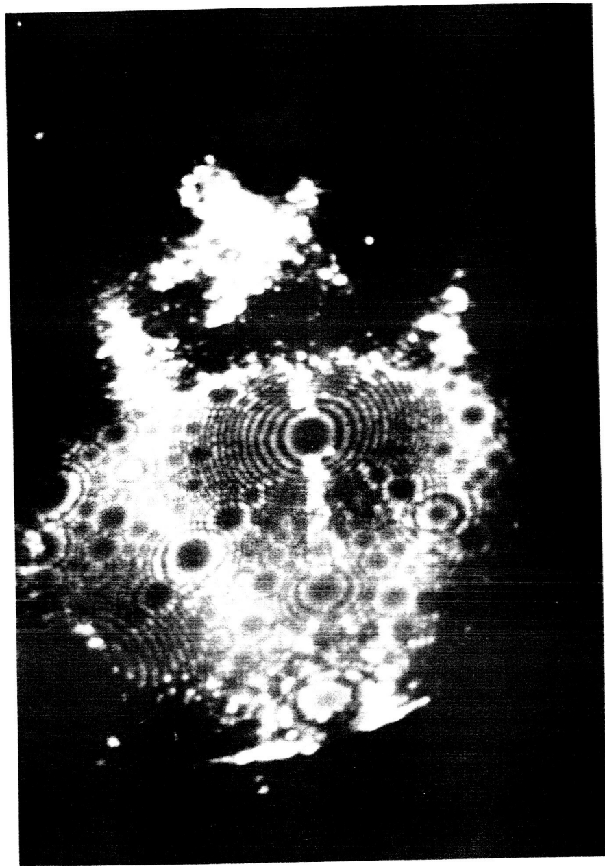
Fig. 9b. Same tip as in Fig. 9a after annealing between 1400^{\circ} - 1600^{\circ}\text{C} for a few seconds inside the microscope. Streaks have disappeared.
