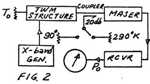
The 20 db directional coupler and the two loads at 90°K and 290°K, respectively, permitted calibration of the system.
