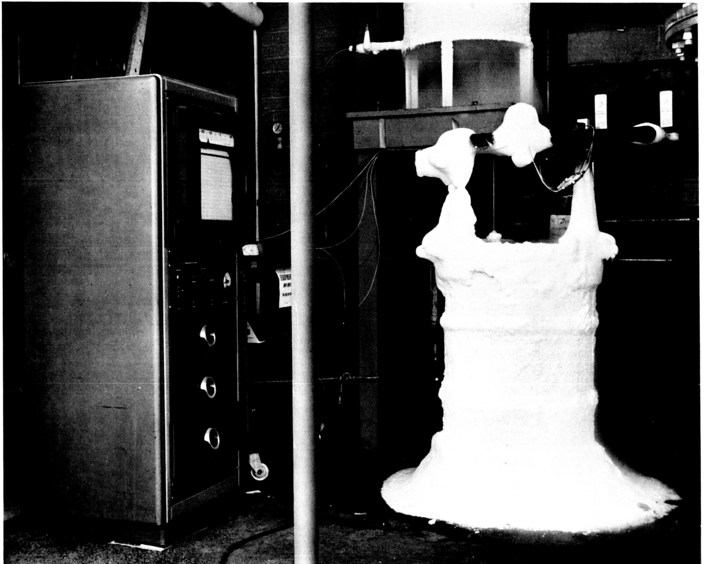
Fig. 2. Refrigerant-valve test setup showing icing conditions
