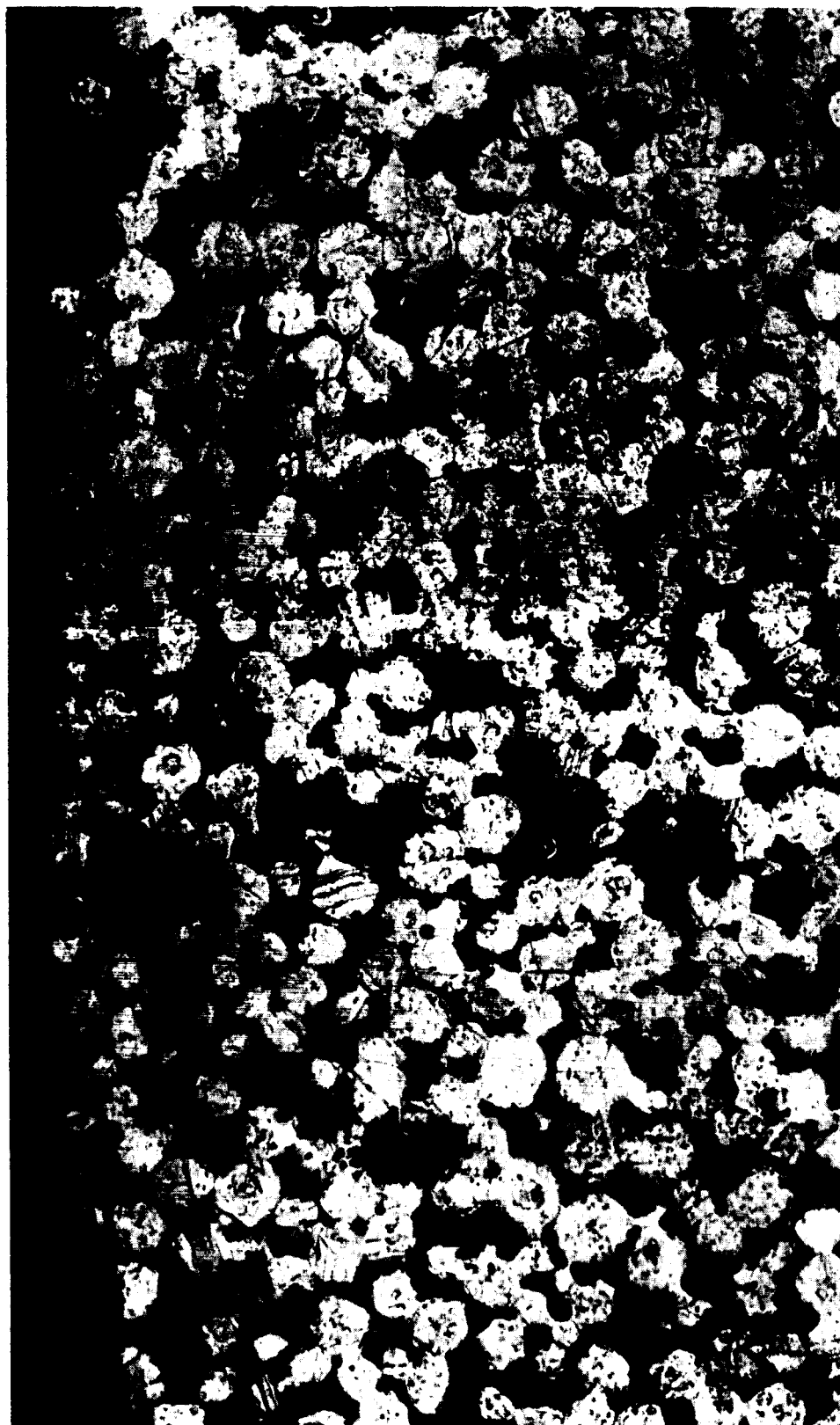
Fig. 25. Composite Map of Porous Anode Surface, Constructed from Photomicrographs. Magnification about 117 diameters.
