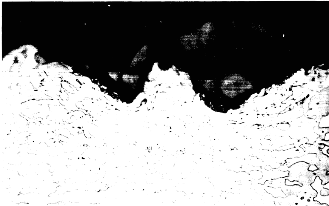
Fig. 29 (a) Transverse Section of Annealed Be-38% Al Extrusion (21-32, 2A-16) Showing Aluminum Segregation (b) Longitudinal Section of Annealed Be-38% Al Sheet (21-31, 2C-5L) Showing Severe Scratches and Imbedded Grit from Grinding Operation
