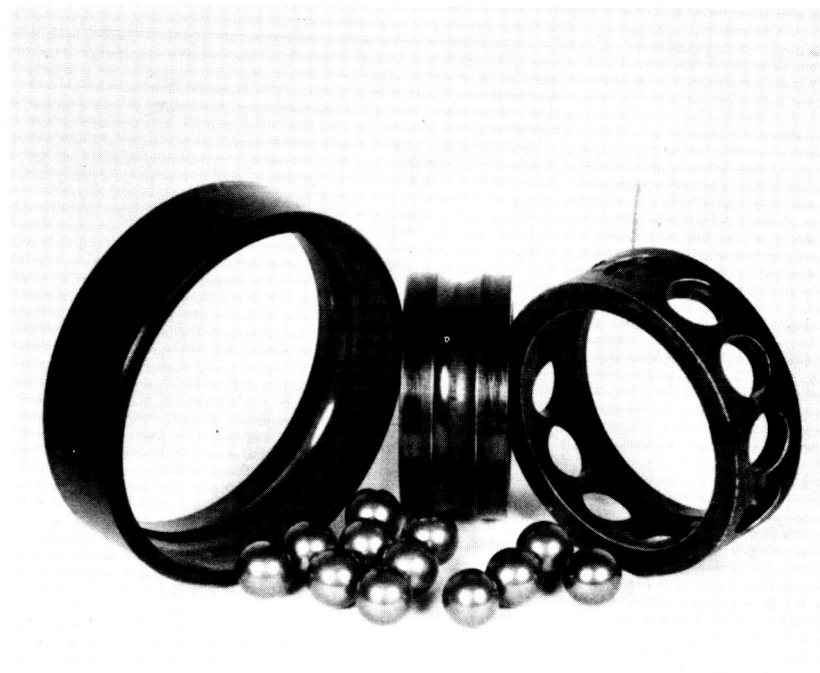
BEARING NO. 392 ON DRIVE END FROM RUN NO. E82
