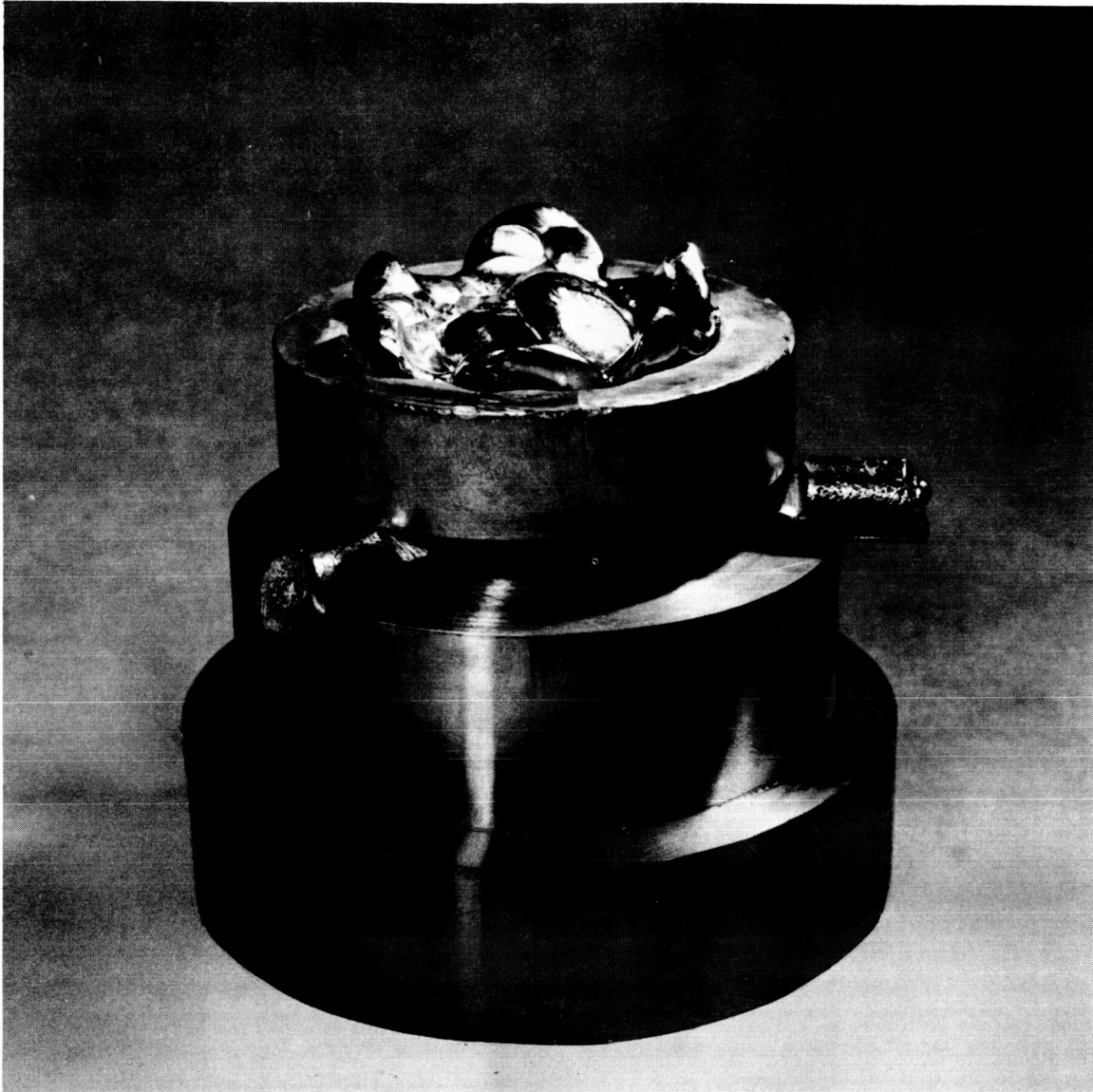
FIGURE 2. APPARATUS FOR DROP CASTING IN THE ELECTRON-BEAM FURNACE
