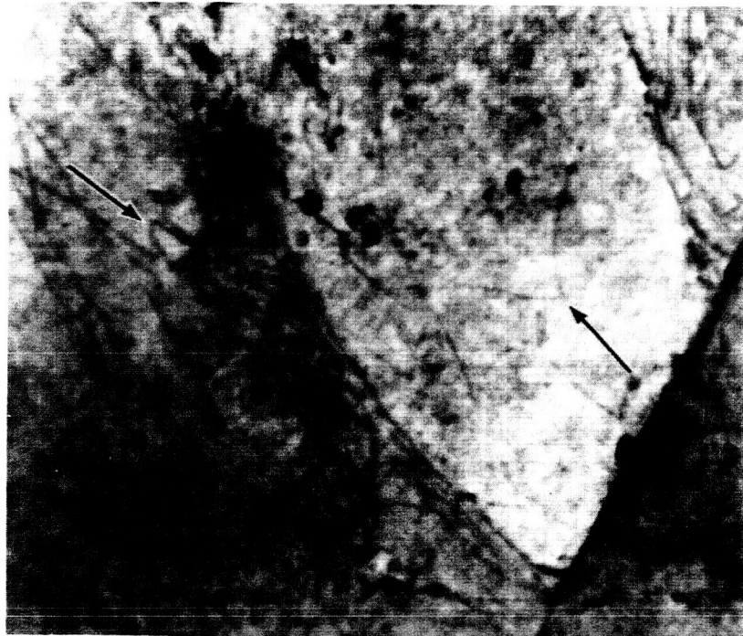
Fig. 3-13 Tensile strained as-received beryllium. Long straight dislocations terminating at a subboundary. Kinked dislocations are arrowed. 40,000: 1
