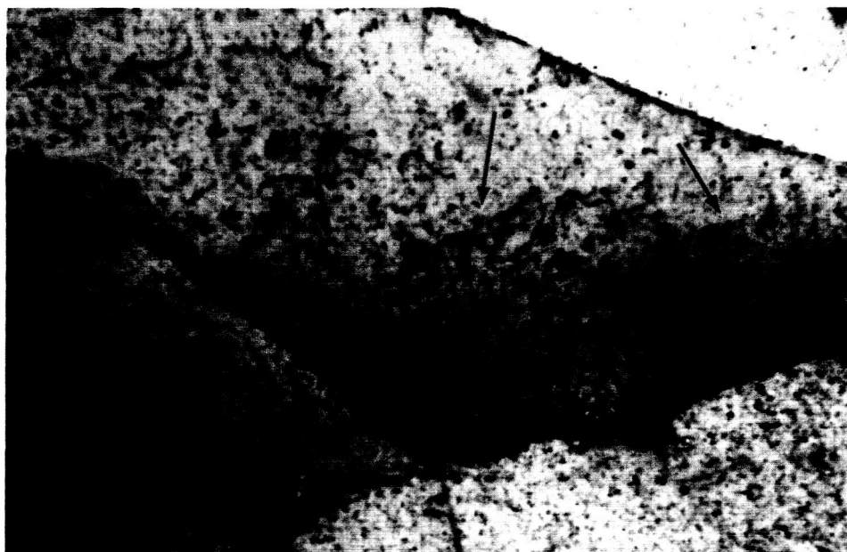
Fig. 3-18 Rows of dislocations making low angle boundaries (arrowed) in annealed beryllium. 40,000: 1
