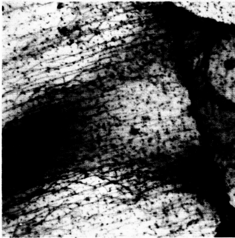
Fig. 3-17 Long parallel dislocation-pairs in annealed and deformed beryllium. 40,000: 1
