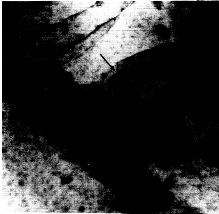
Fig. 3-14 Low angle boundaries (arrowed) and small regions giving rise to contrast effects. Specimen strain-cycled prior to tensile straining. 40,000: 1
