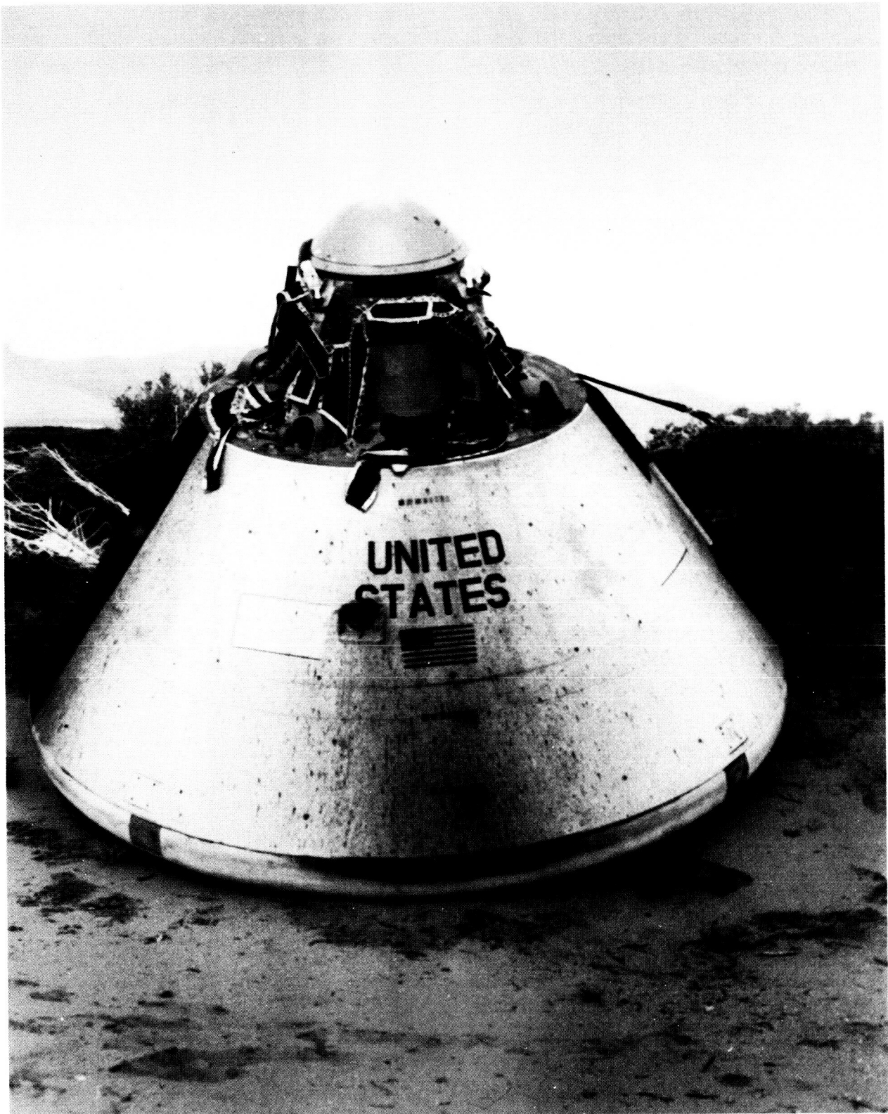
Figure 6. Sooting Due to Solid Products in Jet Exhaust
