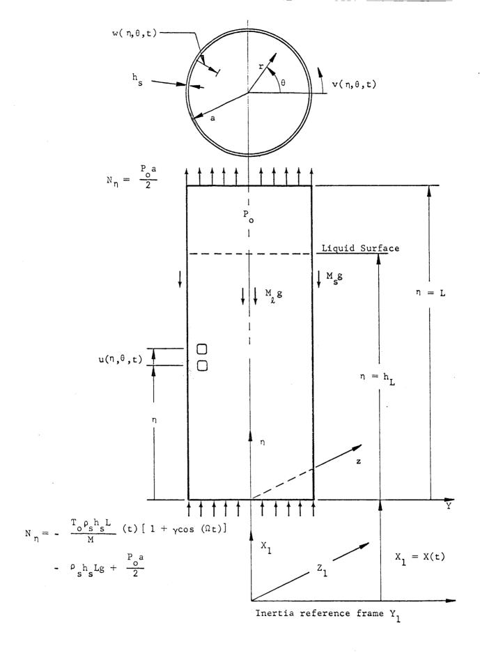
Figure 1 Coordinate System and the Displacement Functions of a Circular Cylinder
