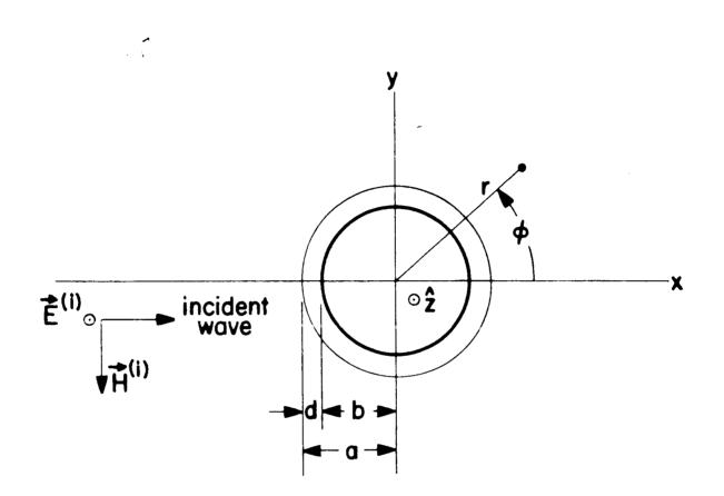
Fig. 1. Basic geometry for the scattering problem.
