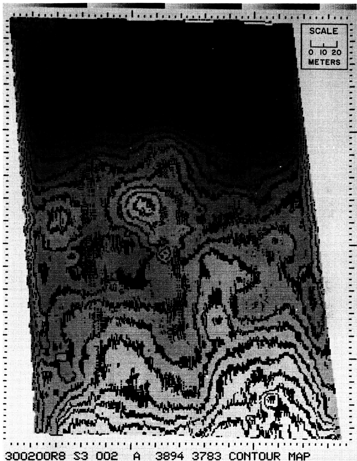
Fig. 8. Rectified contour-map of the same P-3 picture from Ranger VIII (Shading across the frame represents elevation changes, with the convention that, the darker the area, the higher the surface.)
