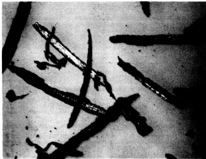
Fig. 4 Shadograph of DX Nickel Fiber
