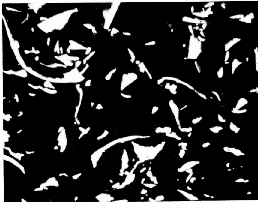
Fig. 6 Photomicrograph of AX2 Nickel fiber sintered plaque 12% dense. Section is perpendicular to felting plane.
