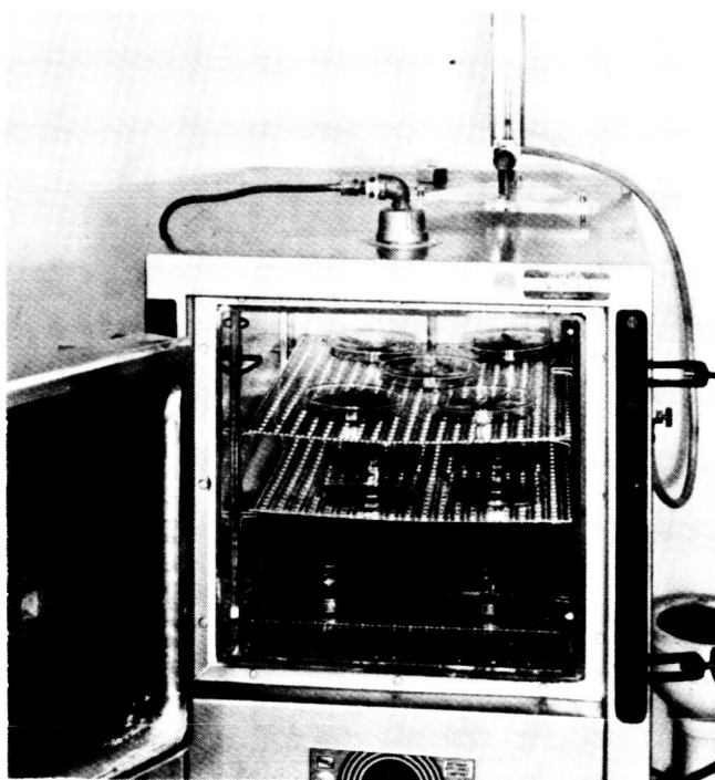
Figure 10. Vacuum oven used for dry heat sterilization tests with weld joints inside (R105391).
