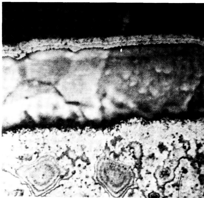
Figure 16. Photomicrographs at 1000X of Specimen F(ii) (gold plated Dumet with nickel undercoat) before and after thermal bake-out. Acetic-nitric etchant.
