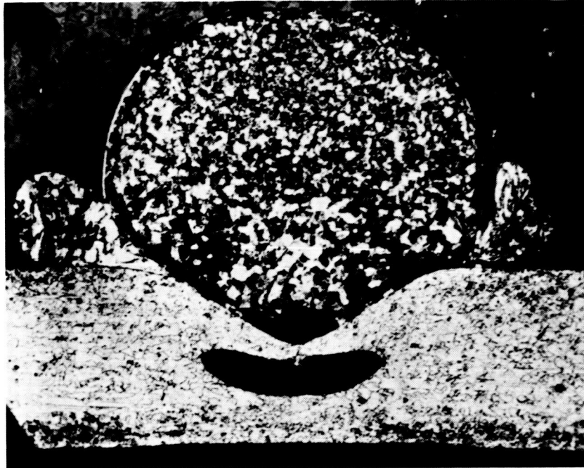
Figure 39. Weld joint 1.5.81; gold plated copper wire to Inco ribbon; not sterilized; 150x magnification; nitric-acetic etch (02332).
