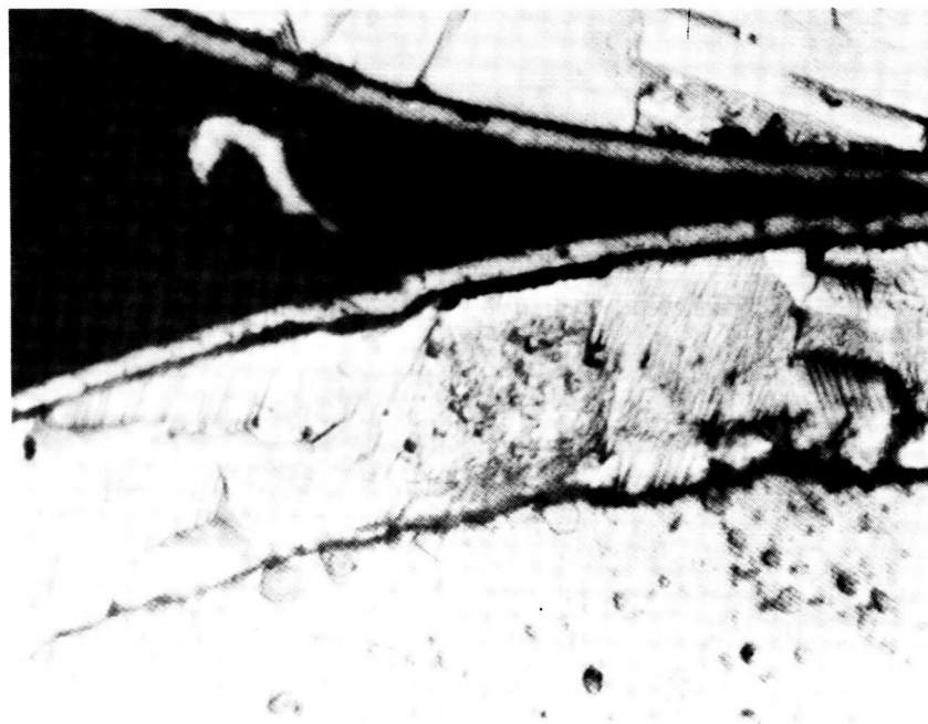
Figure 12. Photomicrographs at 1000X of Specimen B(ii) (gold plated Dumet wire) before and after thermal bake-out. Acetic-nitric etchant.
