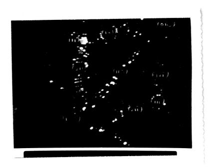
Figure 7 Normal pulse evaporated surface of tungsten showing completely resolved (111) plane with 10 atoms.
