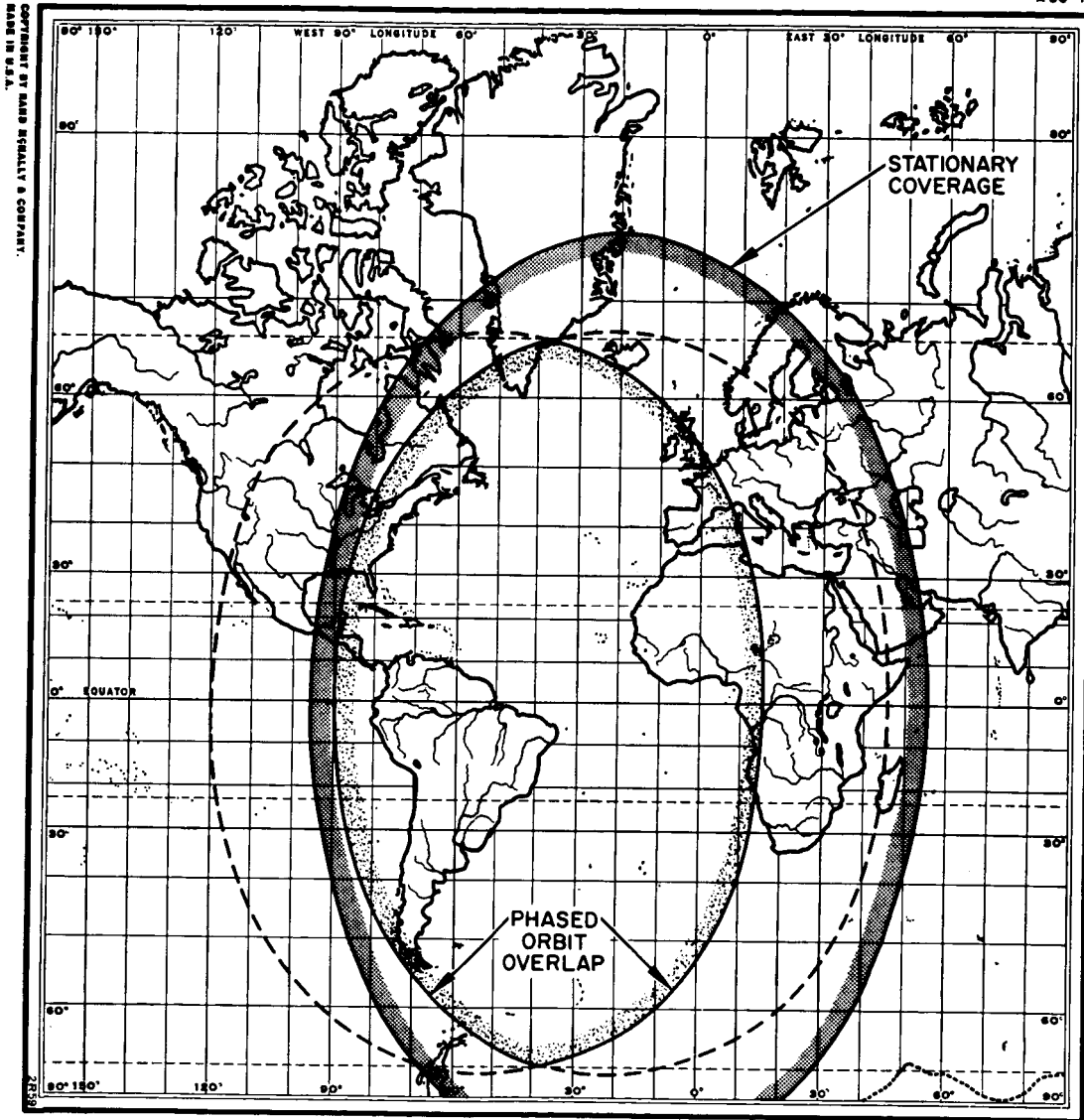
Fig. II-4. Comparison of one-hop multiple access areas for a stationary satellite and for 12 equiphased ( 30^{\circ} separated) 14,000 km equatorial satellites.
