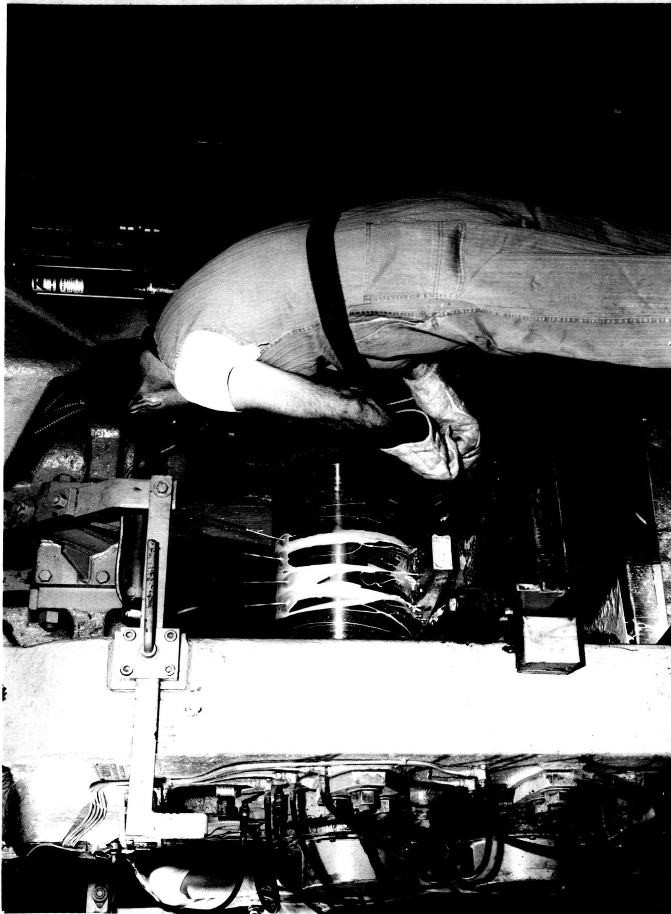
FIGURE 5. SECOND ROLLING PASS ON INGOT FOR 3/4-INCH-THICK PLATE
