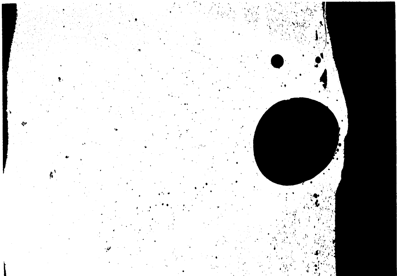
FIGURE 20. MICROSCOPIC APPEARANCE OF A SECTION THROUGH A LARGE PORE IN A BLISTERED WELD
