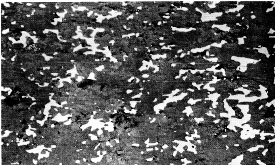
FIG. 9 - MICROSTRUCTURE OF 50 WT% Nb-GRAPHITE (Sample A-4, density = 2.89 g/cc), PRESSED AT 3000°C (320X)
