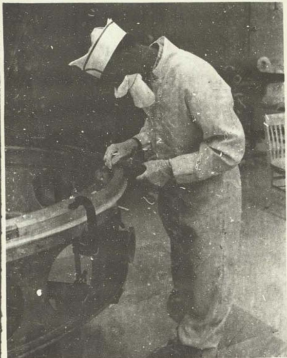
FIGURE 2. APPLICATION OF SILICONE PRIMER.
