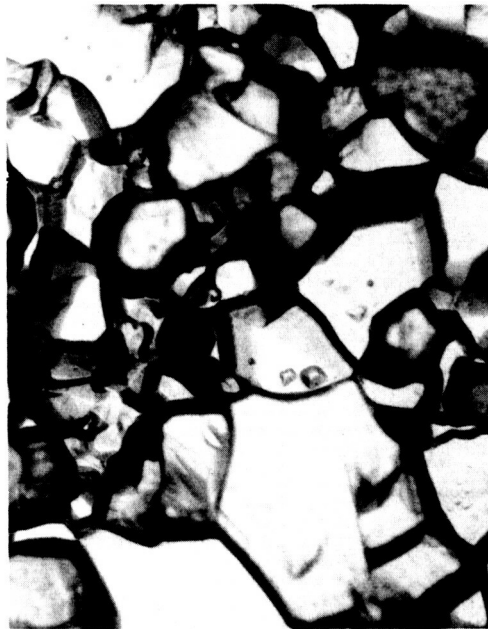
Figure IV-8. Emitter Re31 after Electroetching, 310x.
