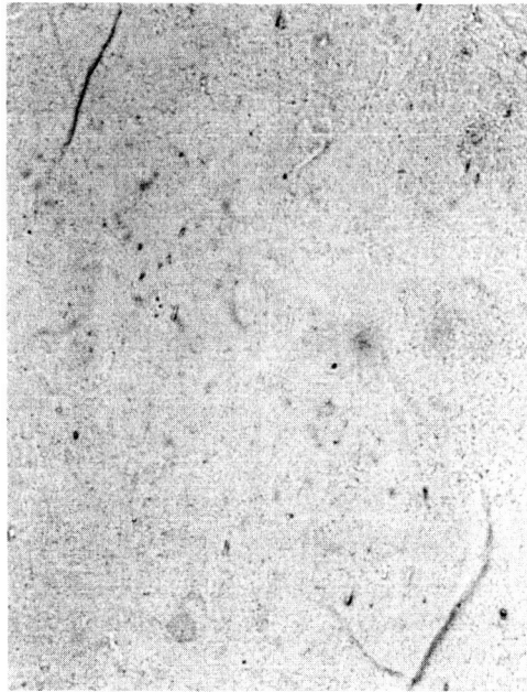
Figure IV -1. Emitter W9 after Electropolishing, 310x.
