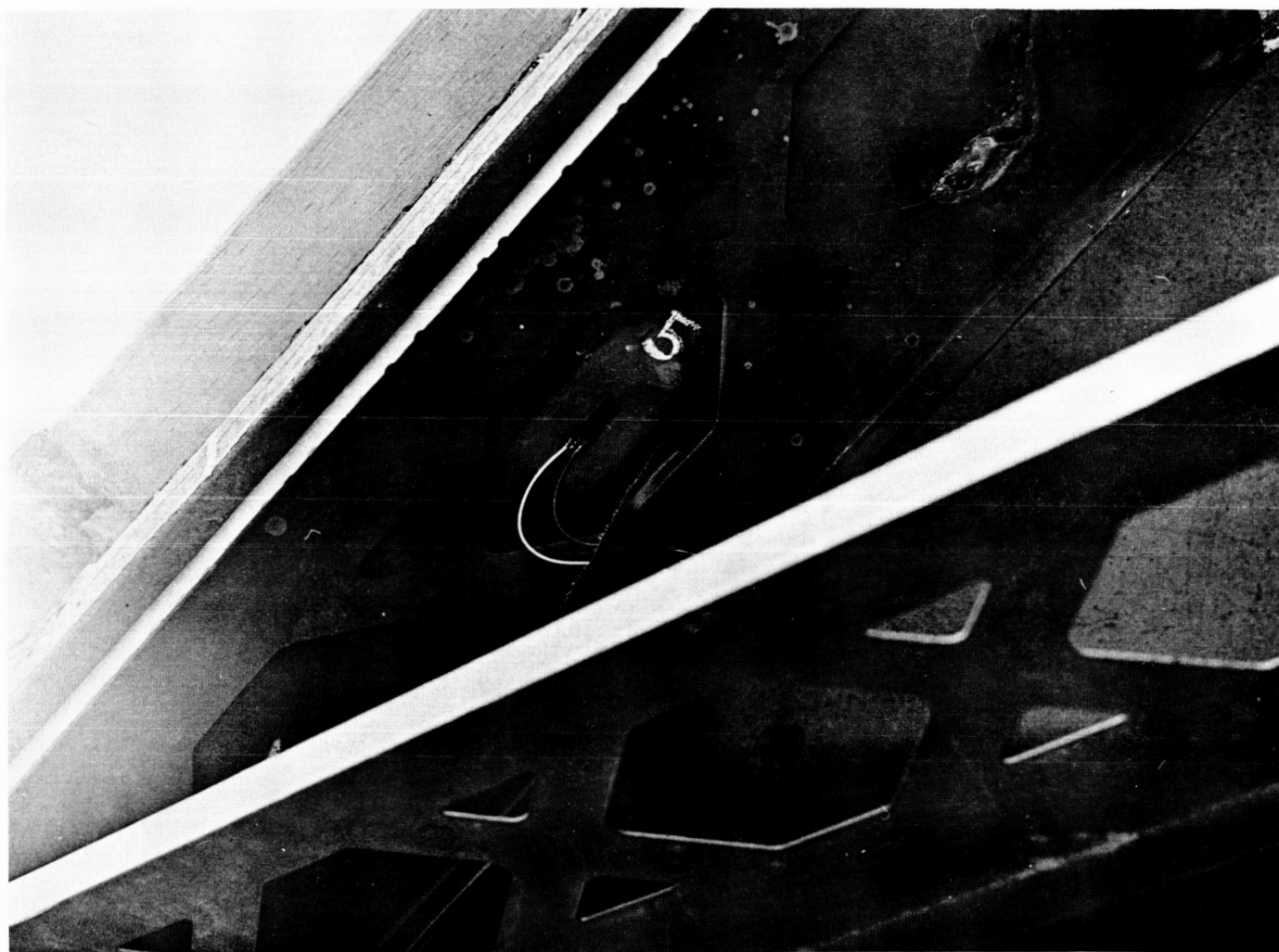
Fig. 8. Strain gauge installation on roof edge on mirror axis of structure
