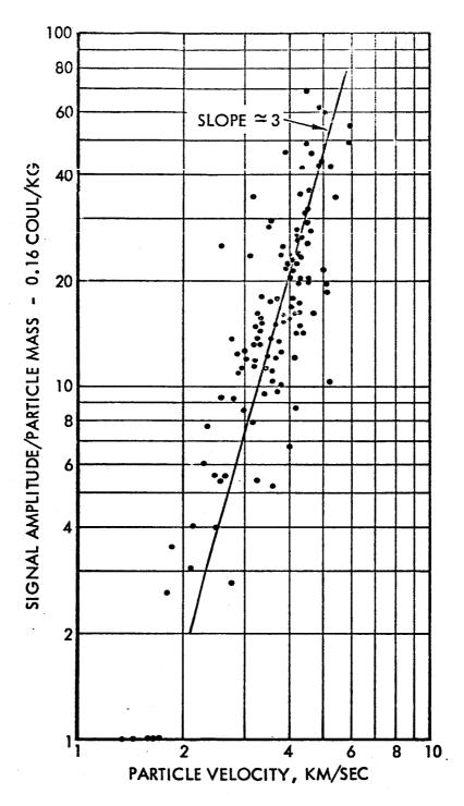
Figure 1. Signal amplitude from semiconductor meteorite detector versus incoming particle velocity.
