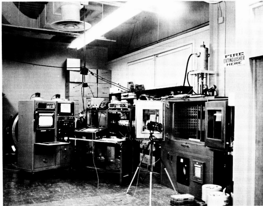
Fig. 21 Hydraulic Ram, Servo Control, Test Frame, Furnace, and Associated Instrumentation for Infinite Plate Study
