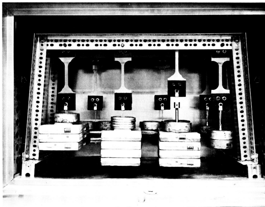
Fig. 7 Loaded Calibration Specimens and Associated Test Frame in Furnace
