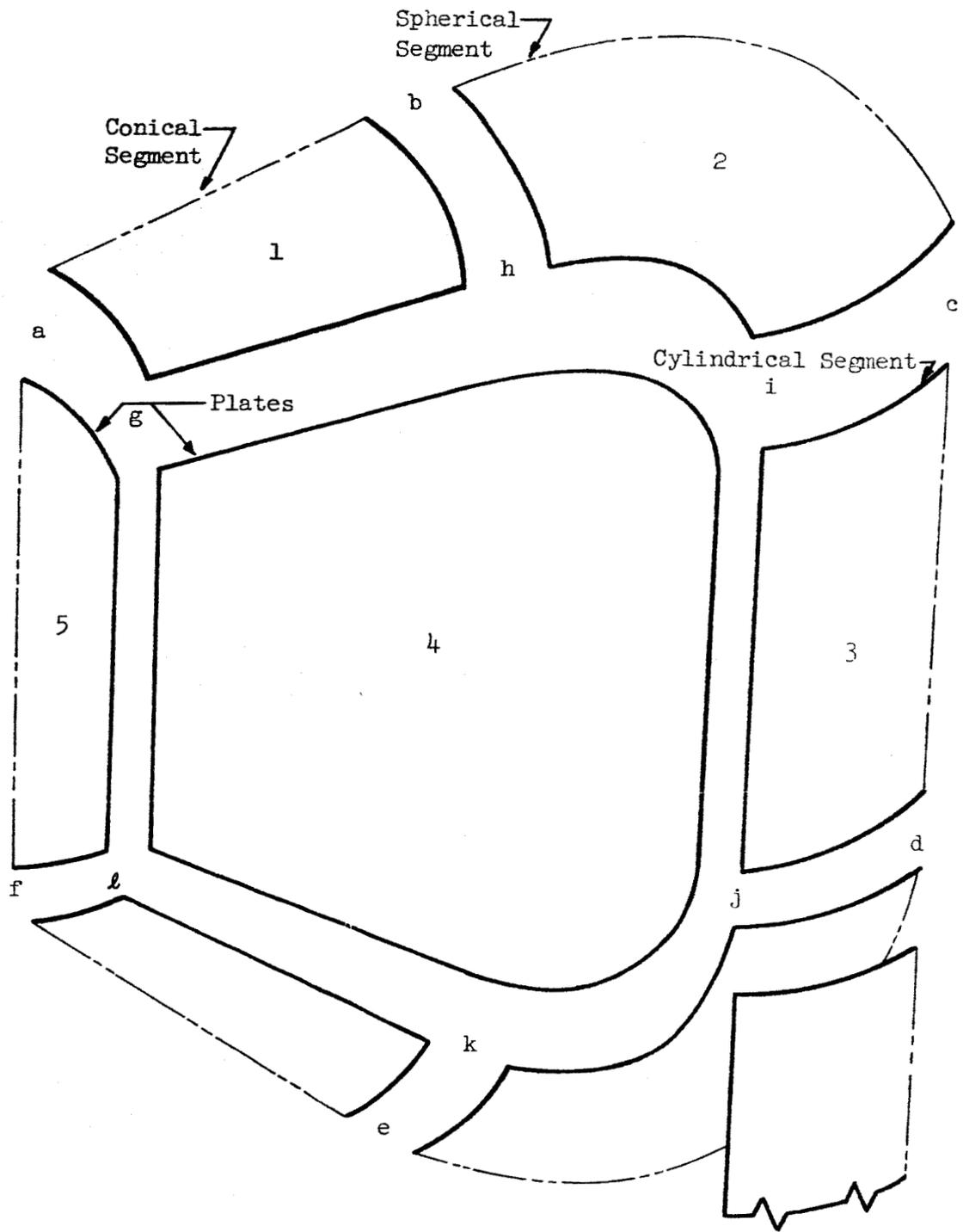
Fig. 2 Basic Shell Elements of Multicellular Structure
