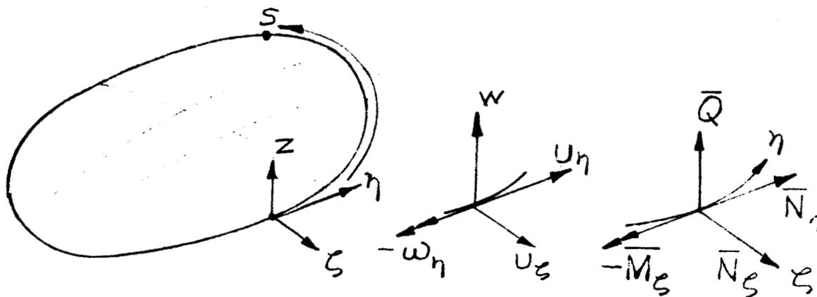
Fig. 3 Boundary Coordinates, Deformations, and Forces
