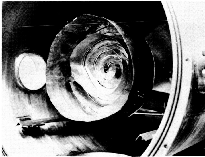
Figure 16. 2ft Diameter x 10" Deep Total Calorimeter Mounted on Movable Base in Vacuum Tank
