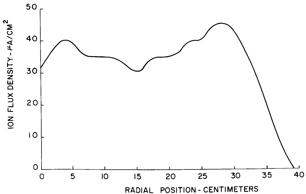
Figure 56. Ion Flux Density Profile Mark V-L Accelerator Argon, .28 mg/sec 2 kw, 3730 Gauss at Window Accelerator-to-Array Distance 70 cm Ambient Pressure 2.5 \times 10^{-5} Torr
