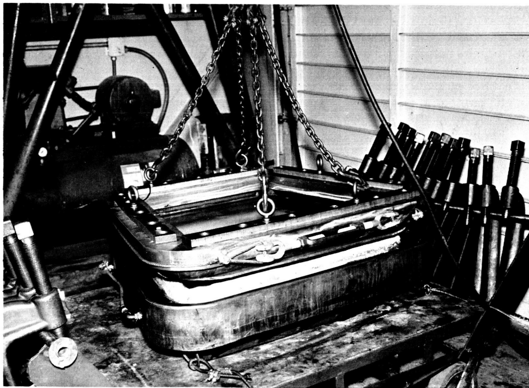
Fig. II-7 Blank and Holddown Bar Alignment
