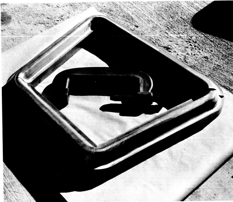
Fig. II-1 Typical C Clamp and Assembled Holddown Bar Used in Explosive Forming
