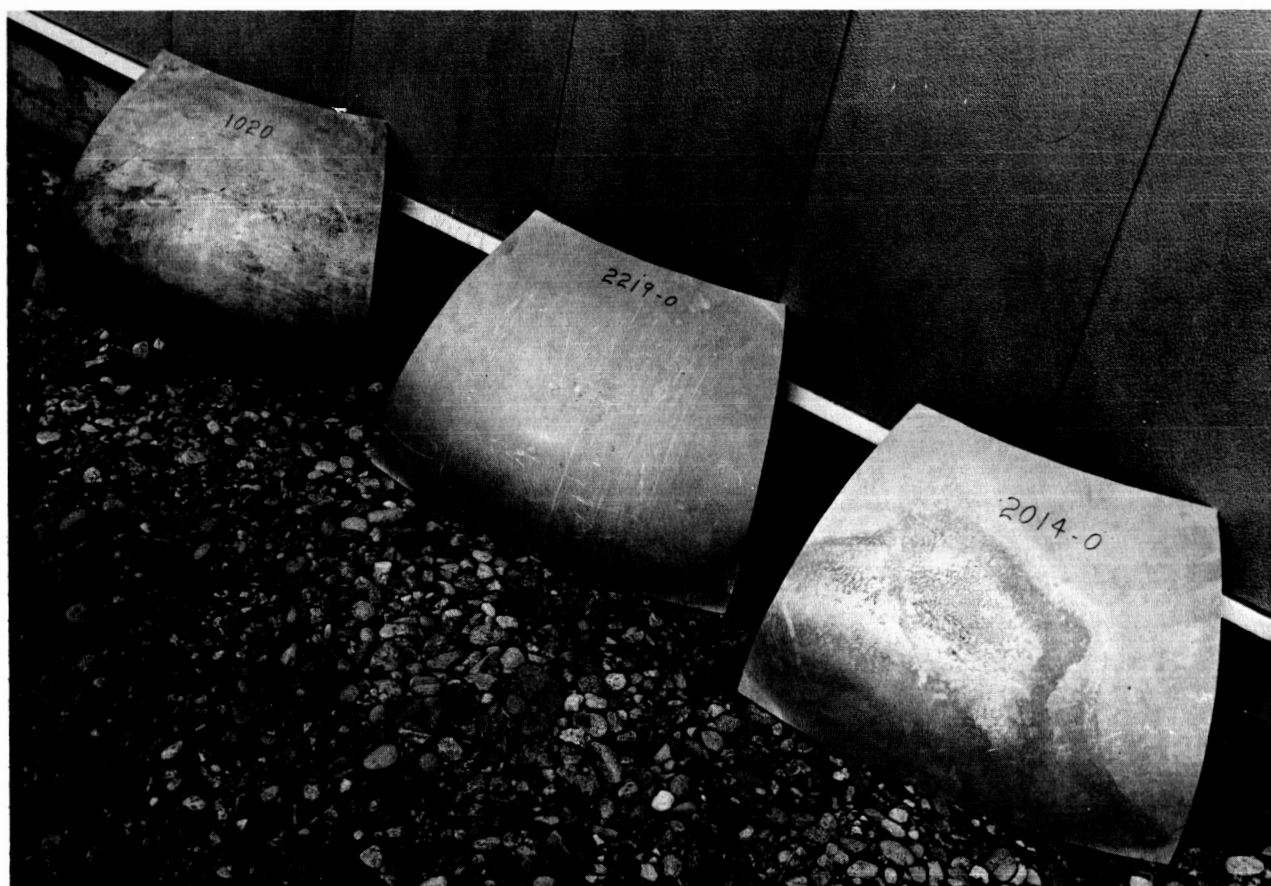
Fig. III-26 Three Segment Parts Explosively Formed
