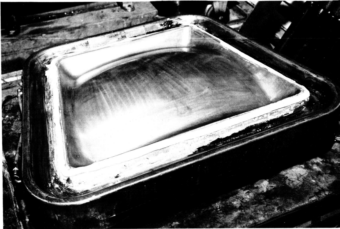
Fig. III-10 Blank Vacuum Sealing with Zinc Chromate Tape
