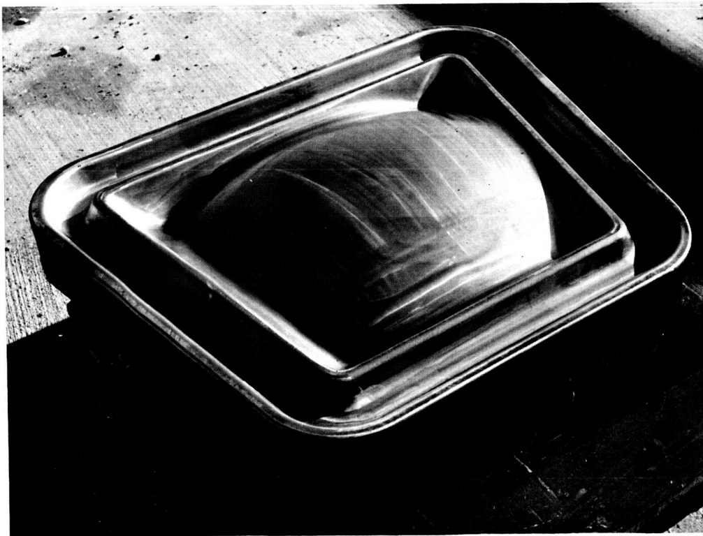
Fig. II-2 Male Forming Die Showing Peripheral Recess Groove
