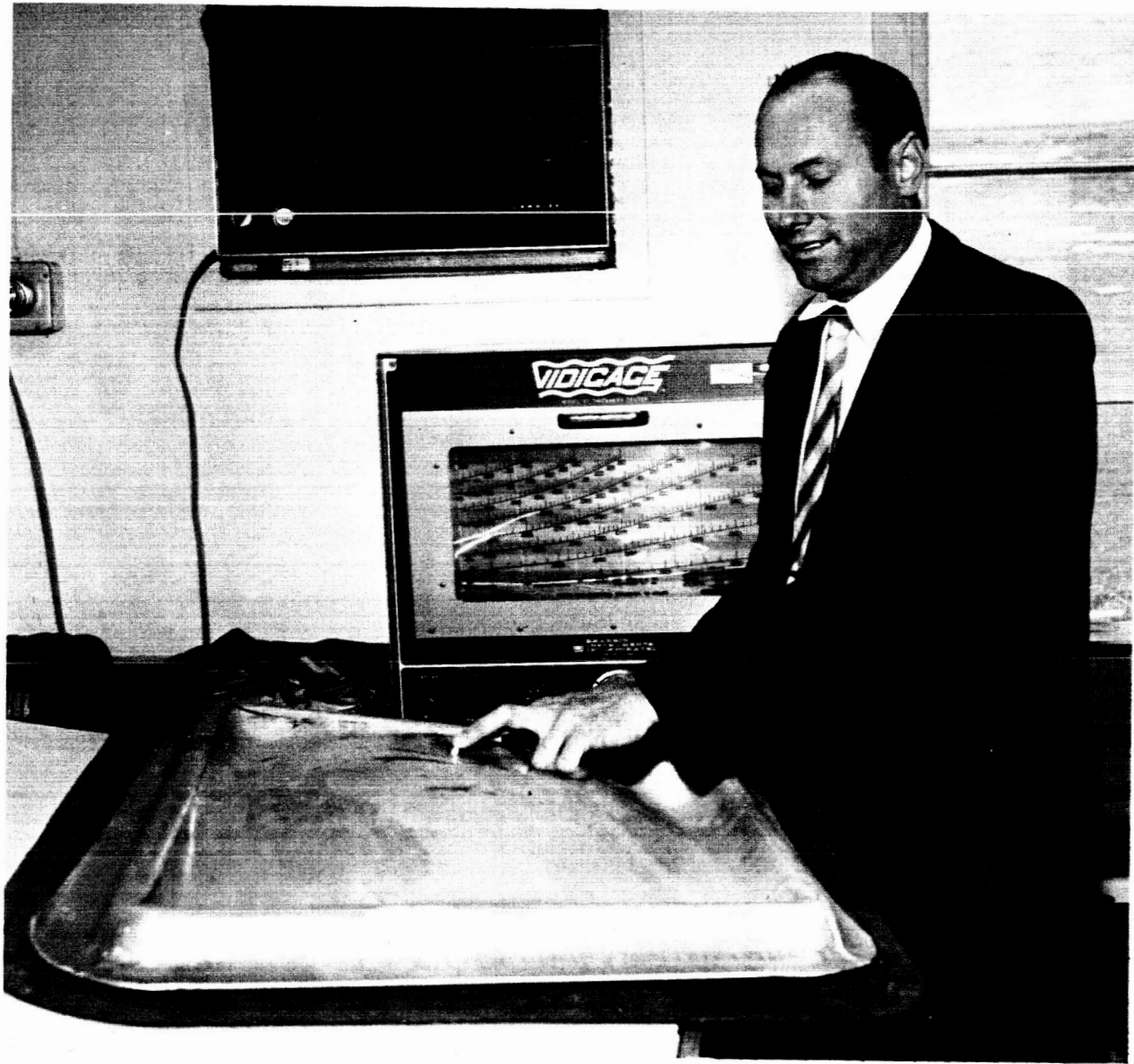
Fig. III-29 Vidigage Thickness Measurements of Explosively Formed Components
