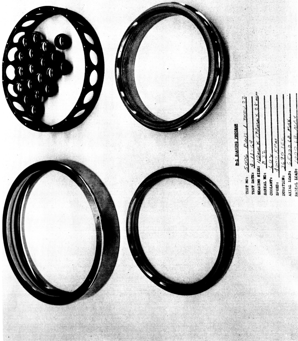
Figure 25 Thrust Bearing, Disassembled (S/N 32B) Page 48
