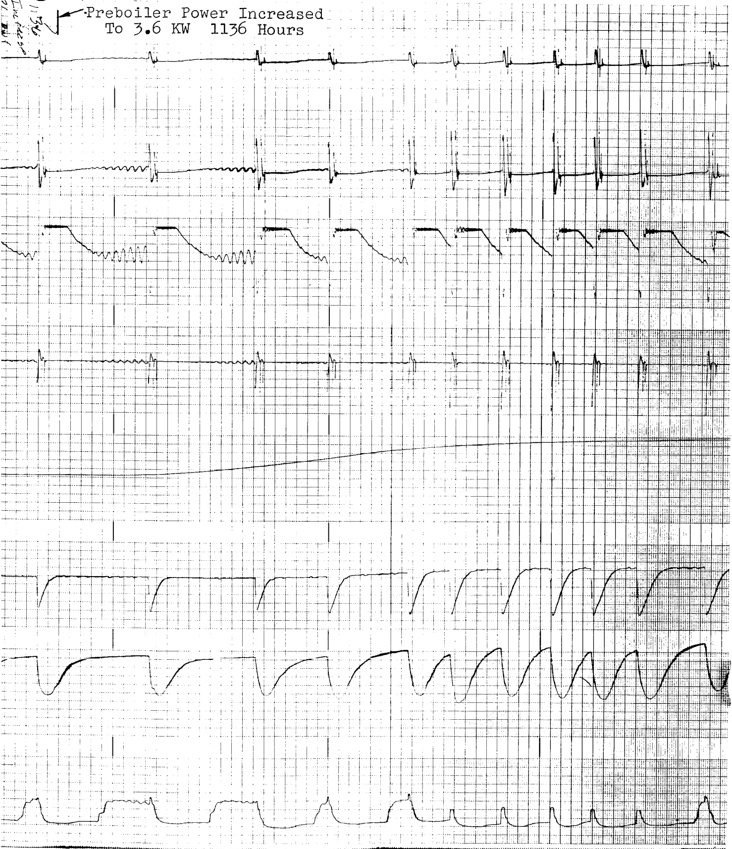
wing Boiling Inception at P = 80 psia. (Continued From Figure 23c) Test Section No. 3).
