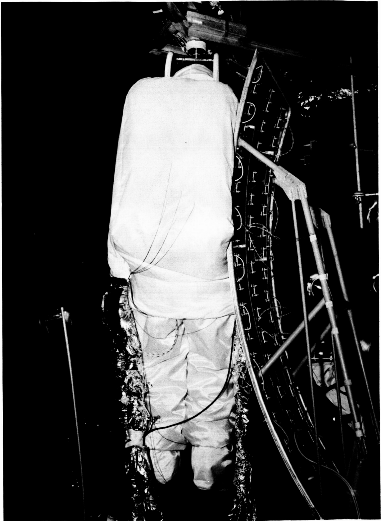
FIGURE 10 SPACECRAFT SURFACE SIMULATOR IN CONTACT WITH SPACE SUIT (EXP. II-A)
