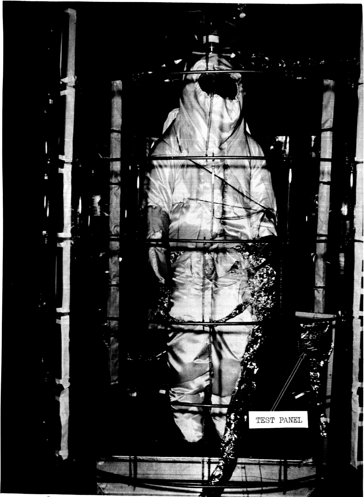
FIGURE D2 BACK OF THERMOCOUPLE TEST PANEL AS MOUNTED IN SES TEST CHAMBER
