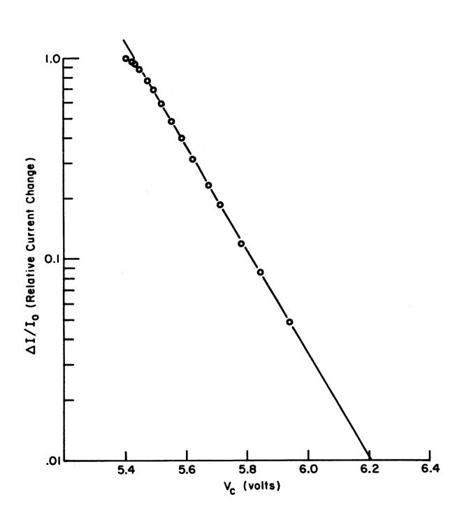
Figure 3. Plot of  $\log \Delta I/I$  vs. tip-to-collector bias voltage according to equation (3) for a 310 oriented tungsten emitter. Anode voltage 1454 volts.
