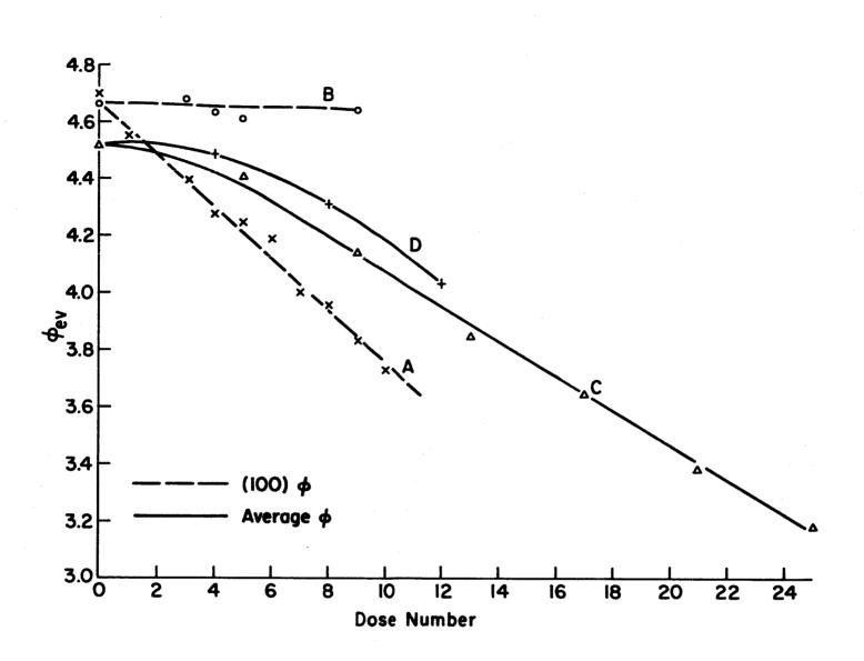
Figure 2. Work function change versus dose number for the 100 planes (curves A and B) and for the average of all planes (curves C and D).
