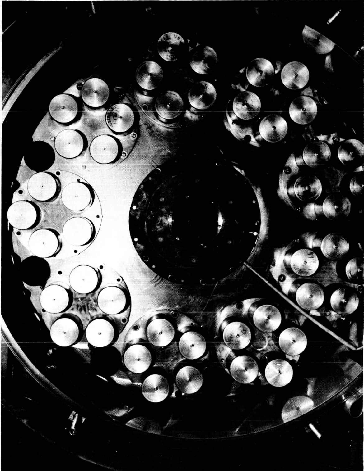
Figure II-5. Capacitor Bank - 42" Overall Diameter
