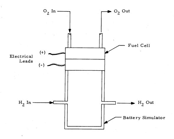
Figure 6. Schematic Diagram of Open Flow Tests
