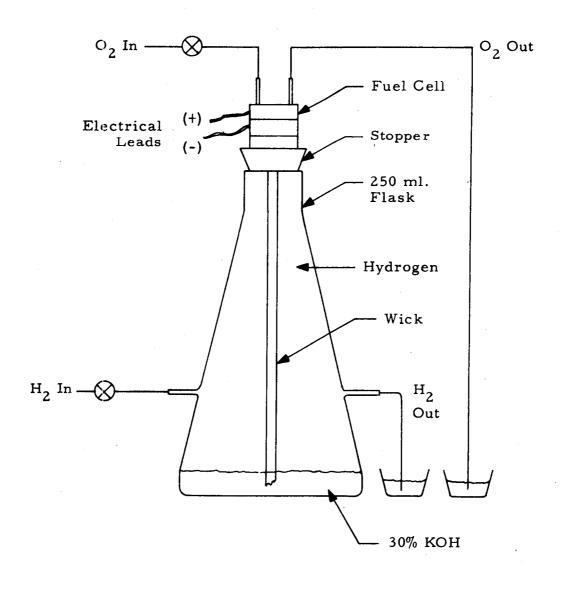
Figure 7. Schematic Diagram of Dead End Flow Tests with Wicks
