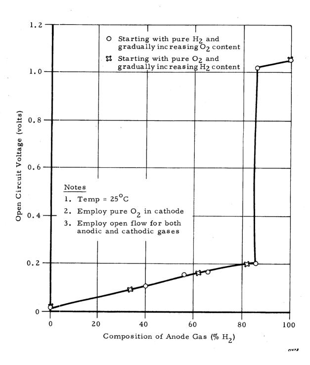
Figure 9. Effect of Composition of Anode Gas on Open Circuit Voltage of H<sub>2</sub>-O<sub>2</sub> Fuel Cell
