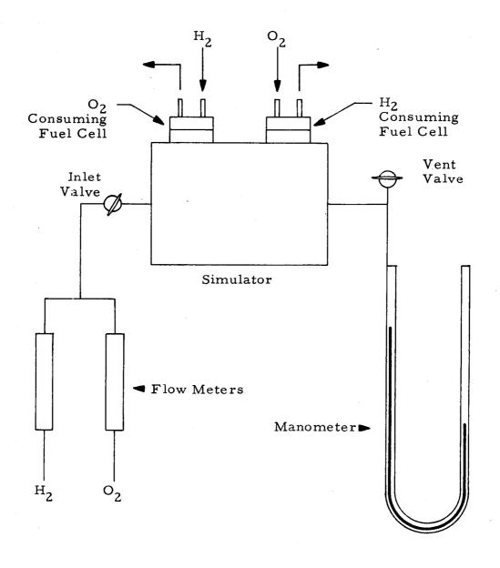
Figure 8. Dual Fuel Cell Arrangement in Battery Simulator
