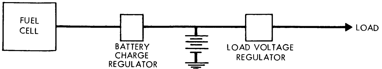
Figure 4-5 POWER SYSTEM CONFIGURATIONS
