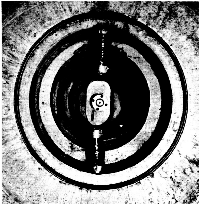
View Looking Into Closed Tank Containing Axial Electrodes of 4" Gap And Kistler #617 Gage Housed In Adapter Assembly
