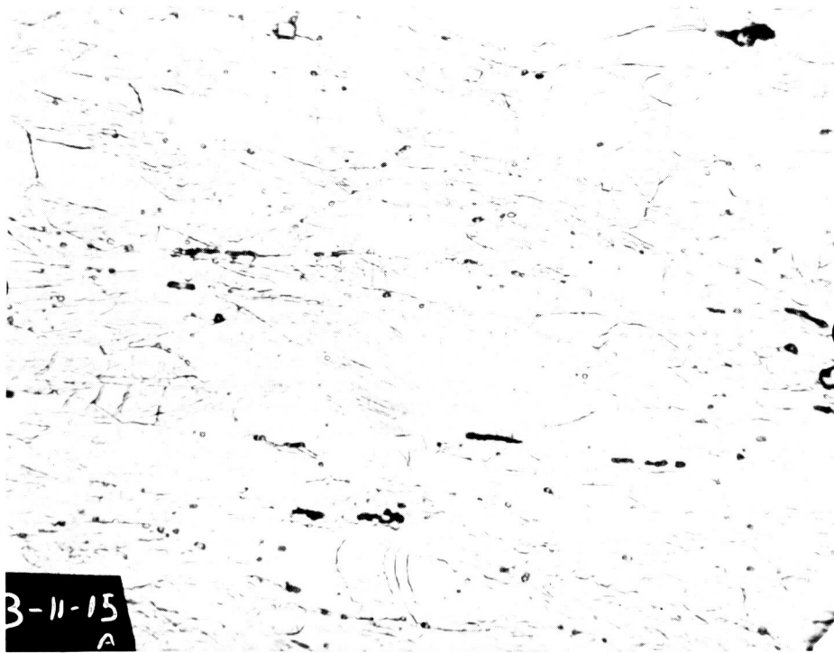
321 STAINLESS STEEL DOME SECTION FORMED TO 48% THINOUT BY THE ELECTROHYDRAULIC PROCESS (HARDNESS: ROCKWELL 15T94)
