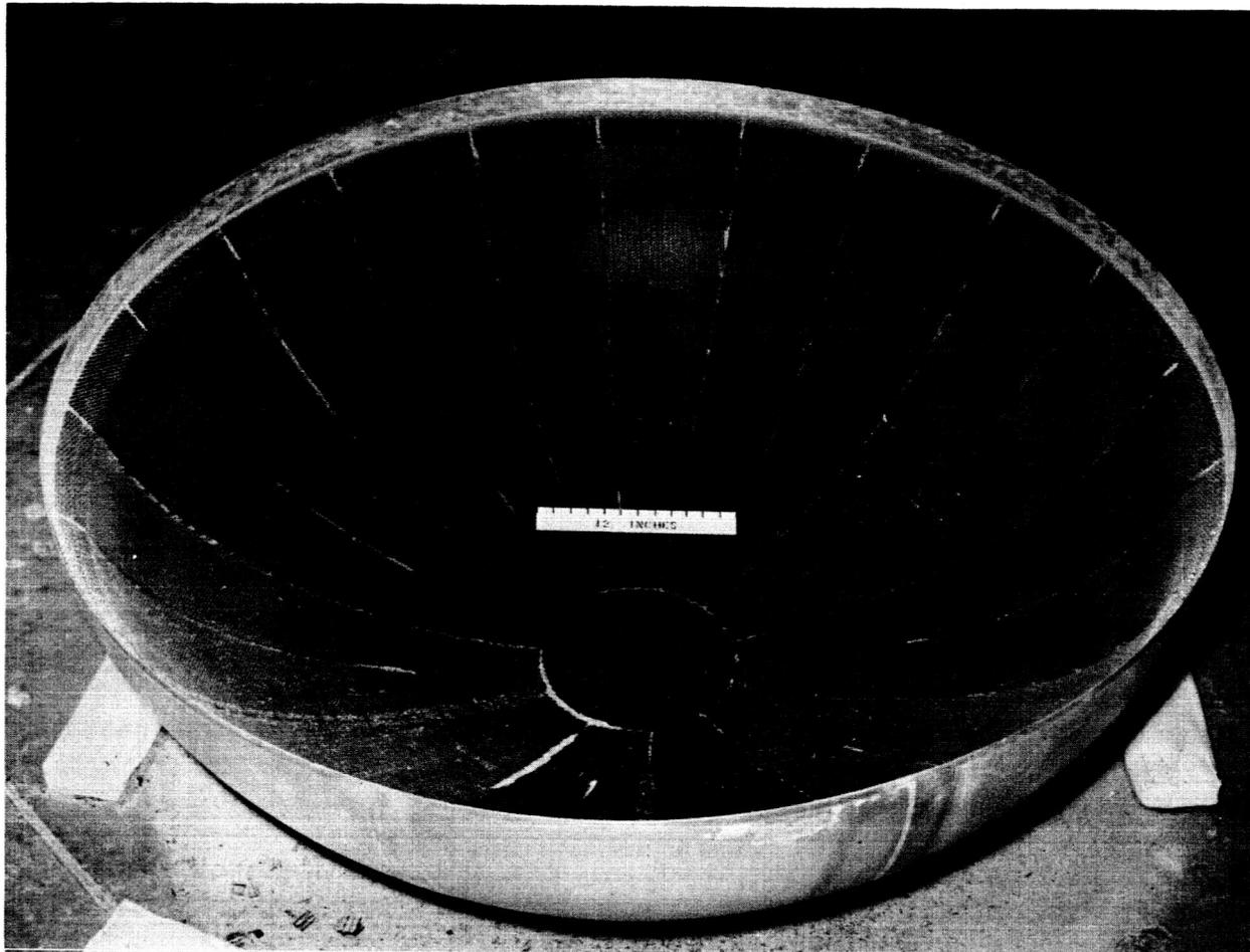
Multipanel Honeycomb Core Prebonded to Outer Skin
