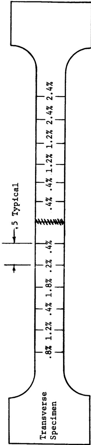
Values noted are percent permanent elongation remaining in each 1/2" increment after application of .8% strain.
