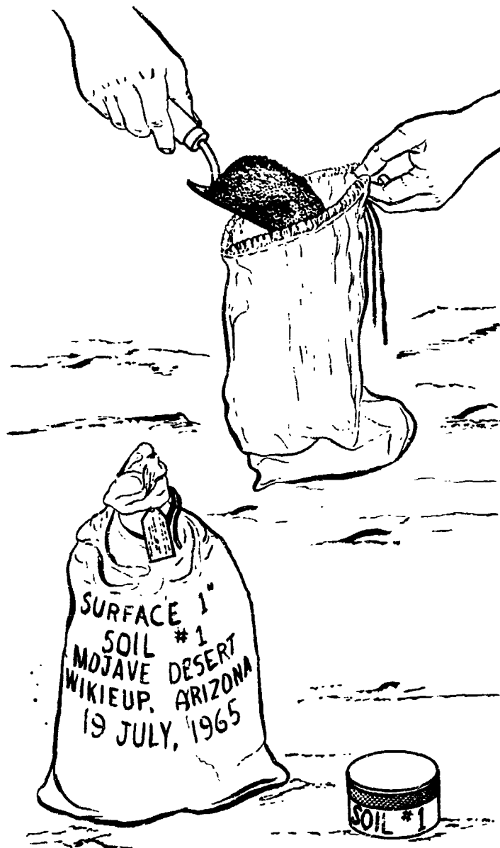
Fig. A-11. Top: sterile sample sack being filled with dislocated soil from sampling site (care is taken not to contaminate the sample during the process of filling the sack); bottom left: properly filled, labeled, and tied sample sack with attached address label (and S-37 soil import authorization form, if necessary); bottom right: properly taped and sealed soil moisture tin containing the same kind of soil as in the sack
