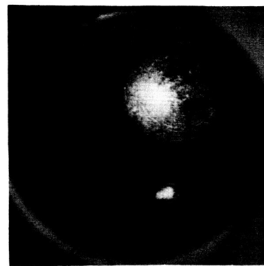
Fig. 27 Oscillating Test. Typical Areas on Bearings Lubricated with \text{MoS}_2 Film Generated by Run-In From Liquid Suspension (Dry Film)
