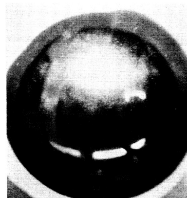
Fig. 25 Typical Contact Areas on Bearings with \text{MoS}_2 Film Generated by Run-In From Liquid Suspension (Dry Film)
