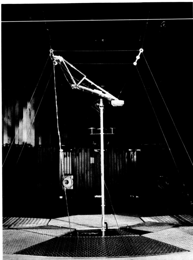
Fig. 15. Surveyor landing leg in the 25-ft space simulator
